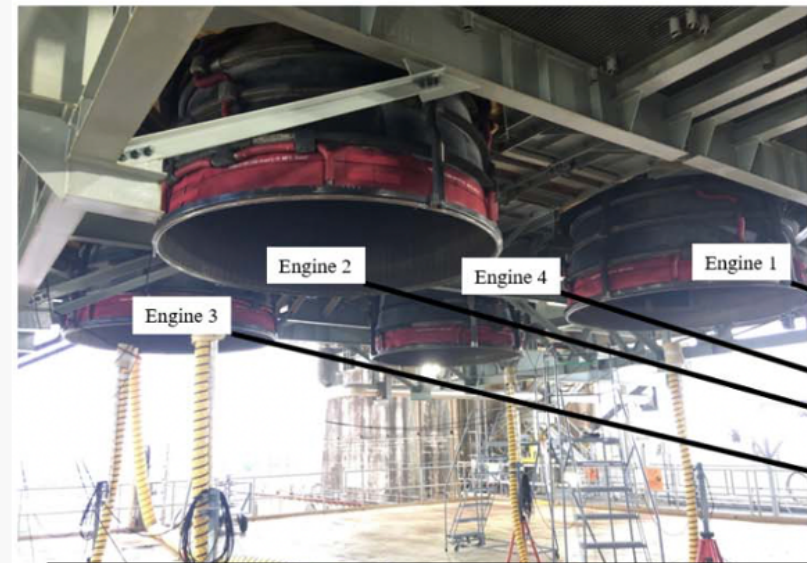
NASA MSFC added accelerometer instrumentation and performed modal ID
