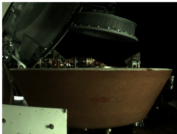
Figure 1: Image of the TAGSAM head being stowed within the SRC on the OSIRIS-REx spacecraft.
