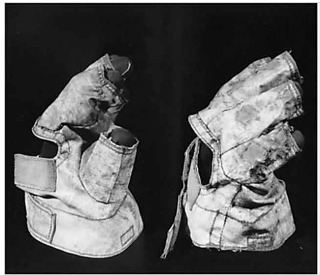
Figure 3. Gene Cernan's worn cover gloves. Note abrasion on right knuckles. [10].
