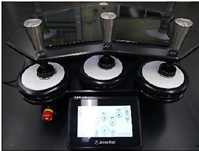
Figure 15. Martindale Model 1605 used in AML at NASA JSC. Circular sample plates are abraded with rotating spindles that hold abrasant grit material.
