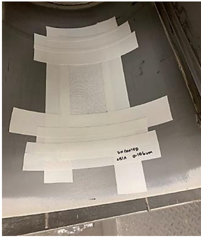
Figure 20. Tumbler set-up before lunar simulant and bean bag were added. Coupon was secured by 2" white Gaffer tape and 3" x 5" inches of Orthofabric were exposed.
