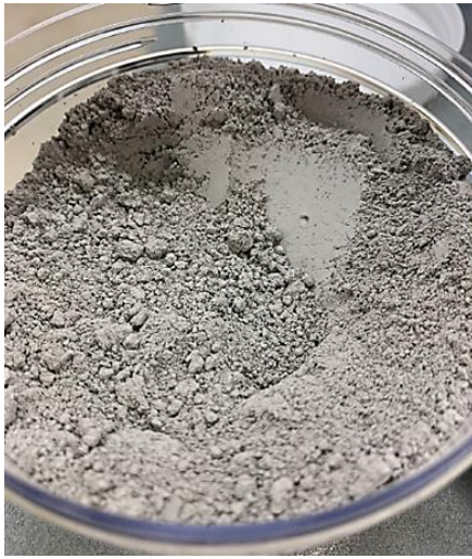
Figure 12. LHS-1D, 0.04 \mu m-35 \mu m. This simulant was not sieved, as it was already at a low enough particle size distribution for testing.
