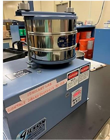
Figure 13. Sieving OB-1A in the Simulant Development Lab.
