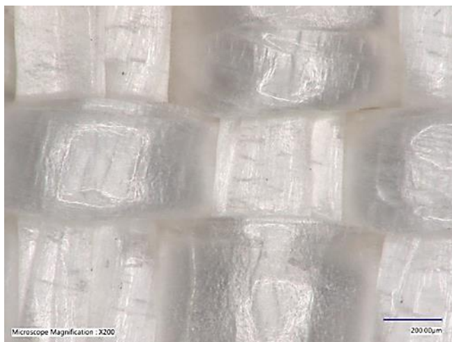
Figure 14. A microscope image of the clean, uncoated Orthofabric bean bag before it was tumbled.
