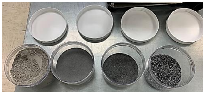
Figure 9. Left to right: LHS-1D 0.04\mu\text{m}\text{--}35\mu\text{m} , OB-1A 0\mu\text{m}\text{--}106\mu\text{m} , OB-1A 106\mu\text{m}\text{--}500\mu\text{m} , and not used but photographed for visual purposes, OB-1A 500\mu\text{m}+ .
