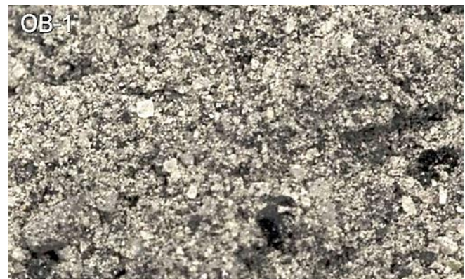
Figure 8. OB-1A consists of Anorthosite (light-colored grains) and olivine slag glass (darker grains) [5].
