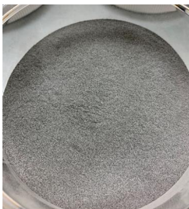
Figure 10. Close-up view of OB-1A, 0\mu\text{m}\text{--}106\mu\text{m} . A fresh batch of simulant was used for each tumble test.
