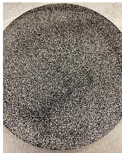
Figure 11. Close-up view of OB-1A simulant, sieved to 106\mu\text{m}\text{--}500\mu\text{m} .
