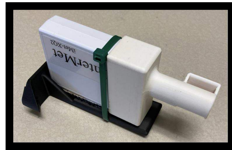
Cover required to account for solar heating affects while maintaining proper ventilation of sensors.
