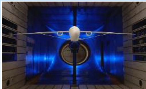
Transonic Truss-Braced Wing 5-10% fuel burn benefit
