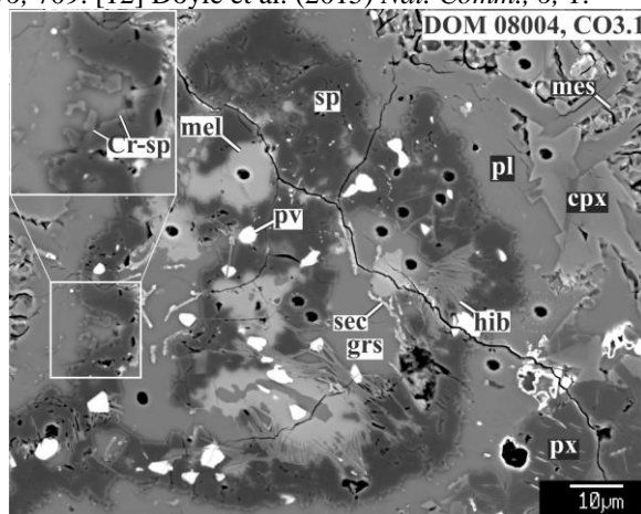
Fig. 3. BSE image of a relict grossite-rich CAI in a porphyritic pyroxene chondrule from DOM 08004 (CO3.1). In Fig. 2b, it is labelled as 2. Cr-sp = Cr-bearing spinel; mes = mesostasis; sec = unidentified secondary phase(s). Holes are SIMS spots.
