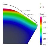
PATO characterization of NuSil coating on PICA in arc jet test conditions – geared to develop better models for recession of MSL and Mars2020
