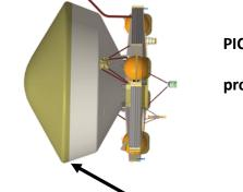
PICA "tooth" design being traded for Dragonfly heatshield to provide protection of main seal – performance assessment requires multi-D capability
