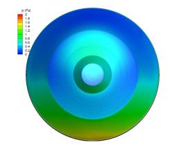
SPARTA used for accurate characterization of Mars2020 backshell and shear stress on woven TPS for MSR-EES to inform spallation
