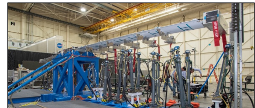
Loads applied using 30 hydraulic actuators
