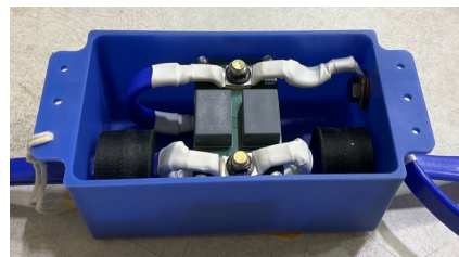
Final filter design is lightweight, compact. Qualified for flight via environmental and system testing.
