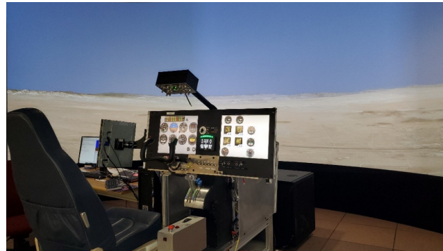
Piloted Sim Cockpit. Pilot seat, Controls, Out-the-Window View, Instrumentation
