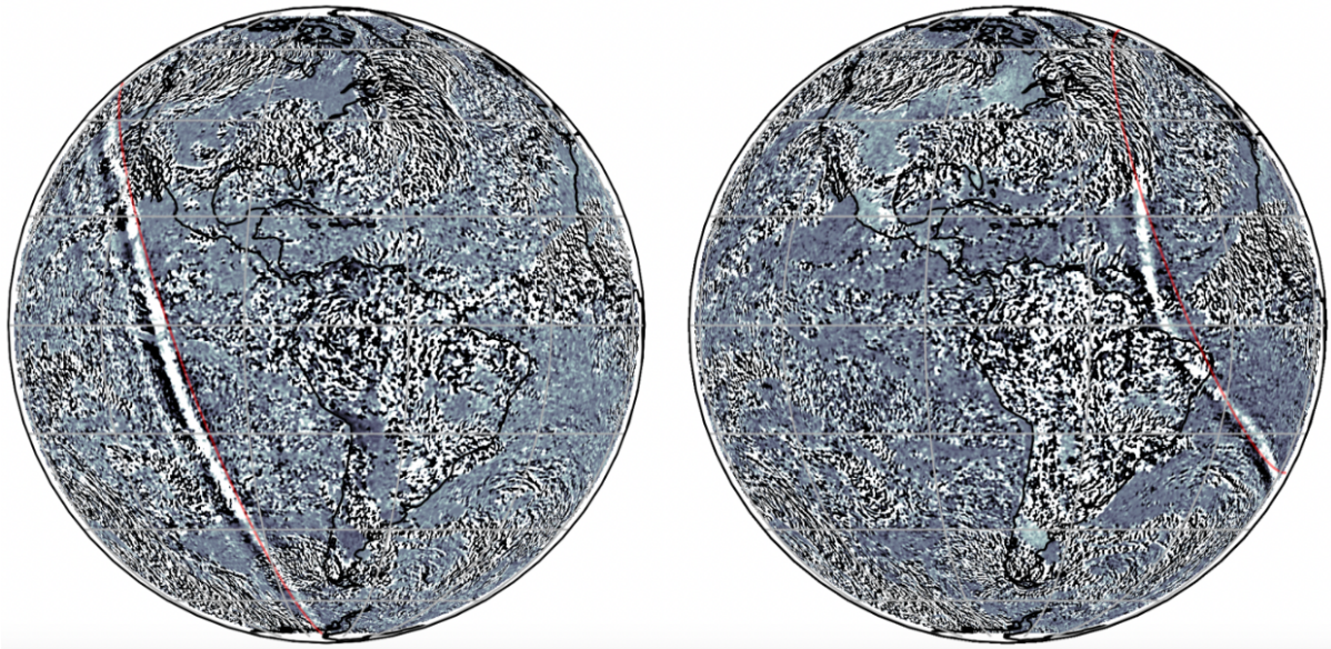
Extended Data Figure 10: The Lamb wave shows evidence of slowing down over South America: Filtered data from GOES' IR channel showing the Lamb wave (strong black/white line) before (left) and after (right) passage over South America. Overlaid red line shows the the expected location of the phase front assuming uniform progression. A deviation from this expected line is seen in the portion of the wave which passed over the northern half of South America.
