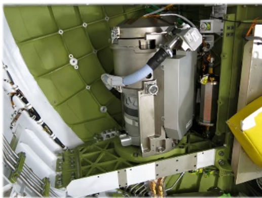
Fig. 1. Orion UWMS installed in Artemis-II Vehicle.
