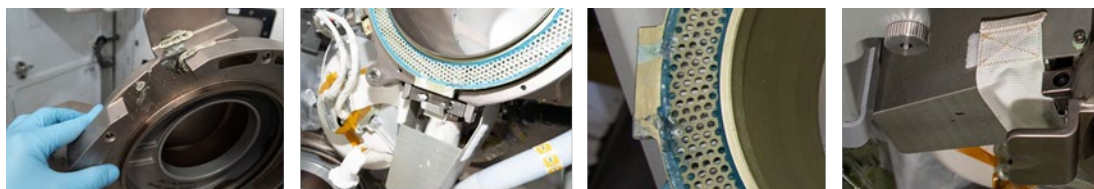
Figure X. Dried residue from pretreat and water solution release on UWMS commode top, access door pins and OBF.
