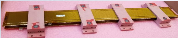
NASA Busbar with MME insulation
