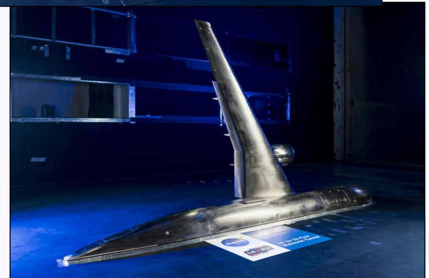
New 5.2% scale CRM-HL model mounted in the 14x22 wind tunnel
