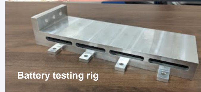
Cu-Mo-Cu enclosure for TMS system testing
