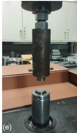
Figure 2.—Experimental equipment (a) MTS 810 test frame, (b) hydraulic grips, (c) specimen alignment, (d) Iosipescu shear test fixture, (e) compression cube fixture, (f) custom fixture for compression tests, (g) CLC compression fixture (top), (h) CLC fixture front showing C2 specimen, (i) Instron 1332 test frame (j) MTS Exceed test frame (k) spring loaded fixture (l) 3-point bend fixture, (m) Two DIC cameras and high-speed camera, and (n) LED lighting fixture.
