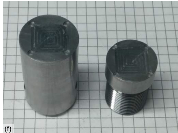
Figure 2.—Experimental equipment (a) MTS 810 test frame, (b) hydraulic grips, (c) specimen alignment, (d) Iosipescu shear test fixture, (e) compression cube fixture, (f) custom fixture for compression tests, (g) CLC compression fixture (top), (h) CLC fixture front showing C2 specimen, (i) Instron 1332 test frame (j) MTS Exceed test frame (k) spring loaded fixture (l) 3-point bend fixture, (m) Two DIC cameras and high-speed camera, and (n) LED lighting fixture.
