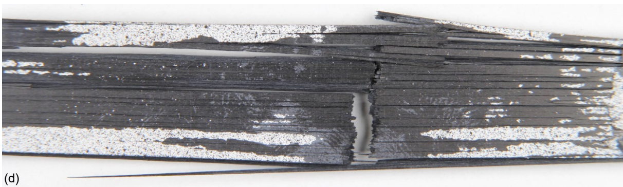
Figure 6.—One-direction tension specimens after testing (a) IM7T1-1, (b) IM7T1-3, (c) IM7T1-4, (d) IM7T1-4 (close-up), (e) IM7T1-5, (f) IM7T1-5 (close-up), (g) IM7T1-6, and (h) IM7T1-6 (close-up).
