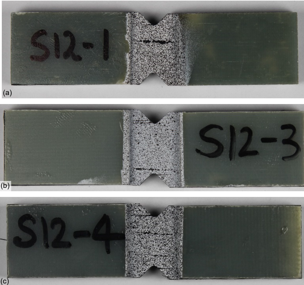
Figure 33.—One-two plane shear specimens after testing (a) IM7S12-1, (b) IM7S12-3, and (c) IM7S12-4.
