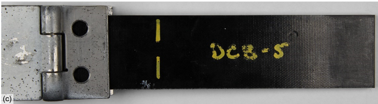
Figure 56.—Image of DCB specimen prior to testing (top surface showing specimen width and side of specimen showing thickness) (a) IM7DCB-2, (b) IM7DCB-3, and (c) IM7DCB-5.
