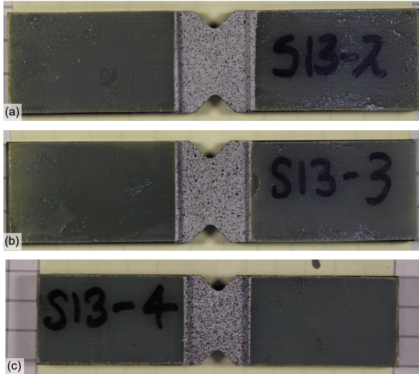
Figure 40.—One-three plane shear specimens prior to testing (a) IM7S13-2, (b) IM7S13-3, and (c) IM7S13-4.
