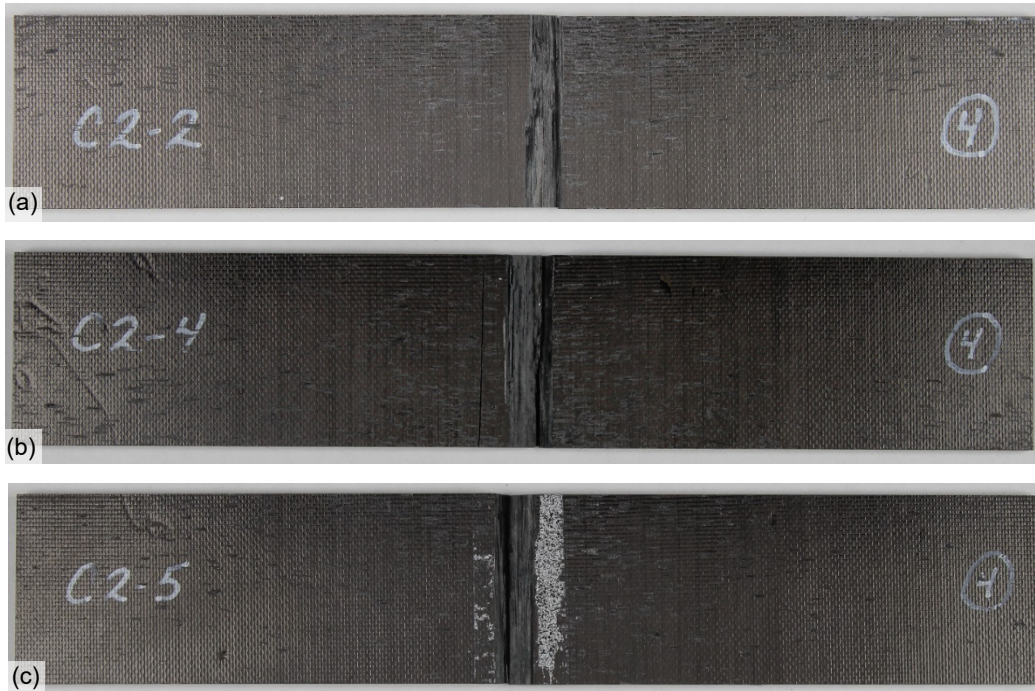
Figure 23.—Two-direction compression specimens after testing (a) IM7C2-2, (b) IM7C2-4, and (c) IM7C2-5.
