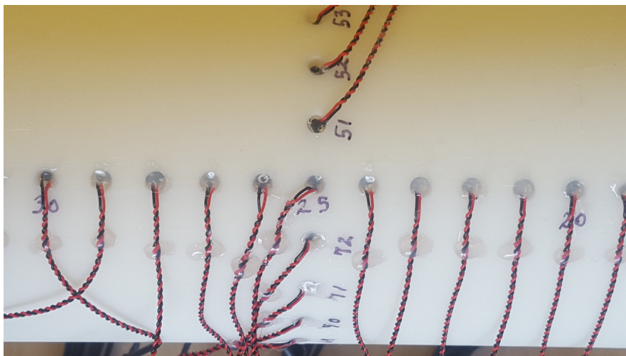
Figure 15.—Microphone array showing installation, numbering, and adhesive.
