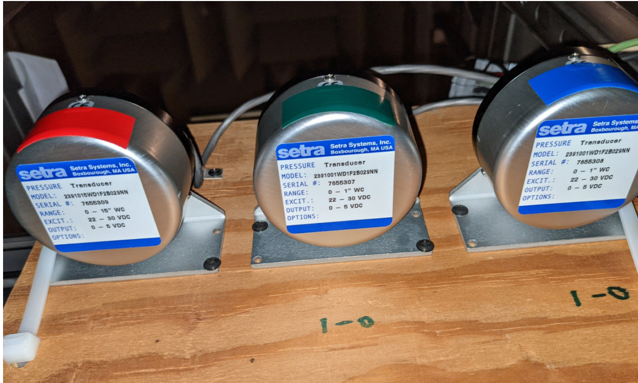
Figure 25.—Setra Model 239 pressure transducers used for testing.
