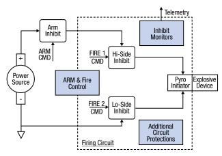
Notional Pyrotechnics Firing Circuit
