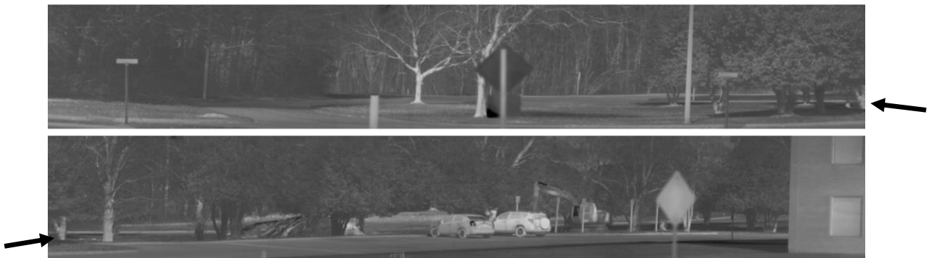
Figure 22. Pushbroom image from the 10.5 \mu\text{m} band of CTI-2. The image was created by repeatedly recording one 1,024-pixel column as the imager was scanned horizontally across the scene. Upper and lower strips are from the same continuous sweep; the rightmost edge of the upper strip overlaps the leftmost edge of the lower strip indicated by the arrows. The frame integration time was 0.5 msec. Lighter gray is higher temperature.
