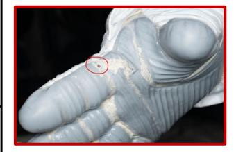
(Dec. 2021) ISS demo of an Al/ML prototype Astronaut glove inspection model that performed diagnostics & generated a GO/NO-GO recommendation in 45 seconds on the glove condition, a process that normally is performed by a group of people taking multiple days.
