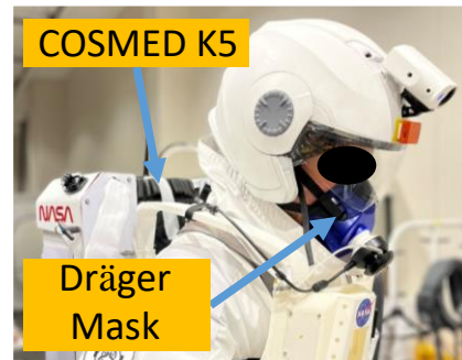
Figure 5. Subject wearing a COSMED system with a Dräger mask underneath the helmet with cables routed to the K5 secured in the PLSS.
