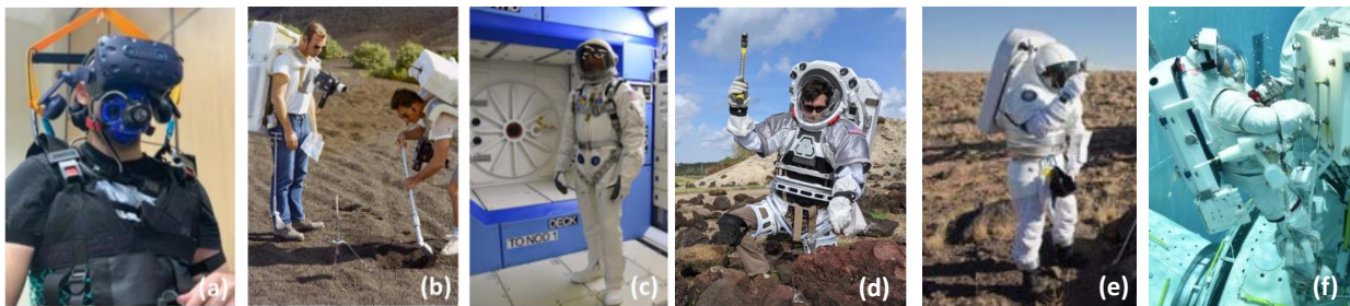
Figure 1. Examples of spacesuit simulators used in human spaceflight. (a) Unsuited analog used in the Assessments of Physiology and Cognition in Hybrid-reality Environments (APACHE) study. 7 (b) Limited interface simulator used by Apollo crew to conduct geological training (source: NASA). (c) Representational simulator used by public affair teams. (d) Unpressurized full-spectrum simulator built by Atlas Devices to provide realistic range of motion, and ergonomic capabilities of the NASA's xEMU suit. 8,9 (e) Unpressurized full-spectrum suit with multiple roll joints used by the Desert Research and Technology Studies (DRATS) . 3,6 (f) Fully pressurized suit (Z-2.5) used in the NASA neutral buoyancy laboratory (NBL) for crew training. 10
