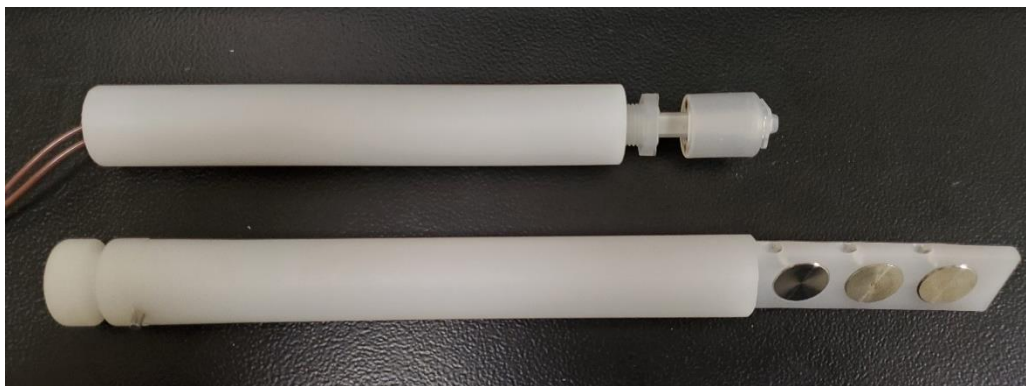
Figure 5: Fabricated Housing for the Float Switch Next to a Coupon Sample Rod
