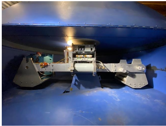
Fig. 3 SRSC #3 prototype installed in the Centrifuge Test Facility located at Case Western Reserve University.
