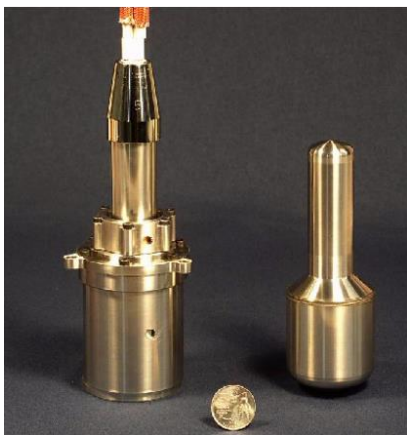
Fig. 6. EE-35 gas-bearing free-piston Stirling prototype (left) and mass model of lightweight flight version (right). Image courtesy of Sunpower, Inc.
