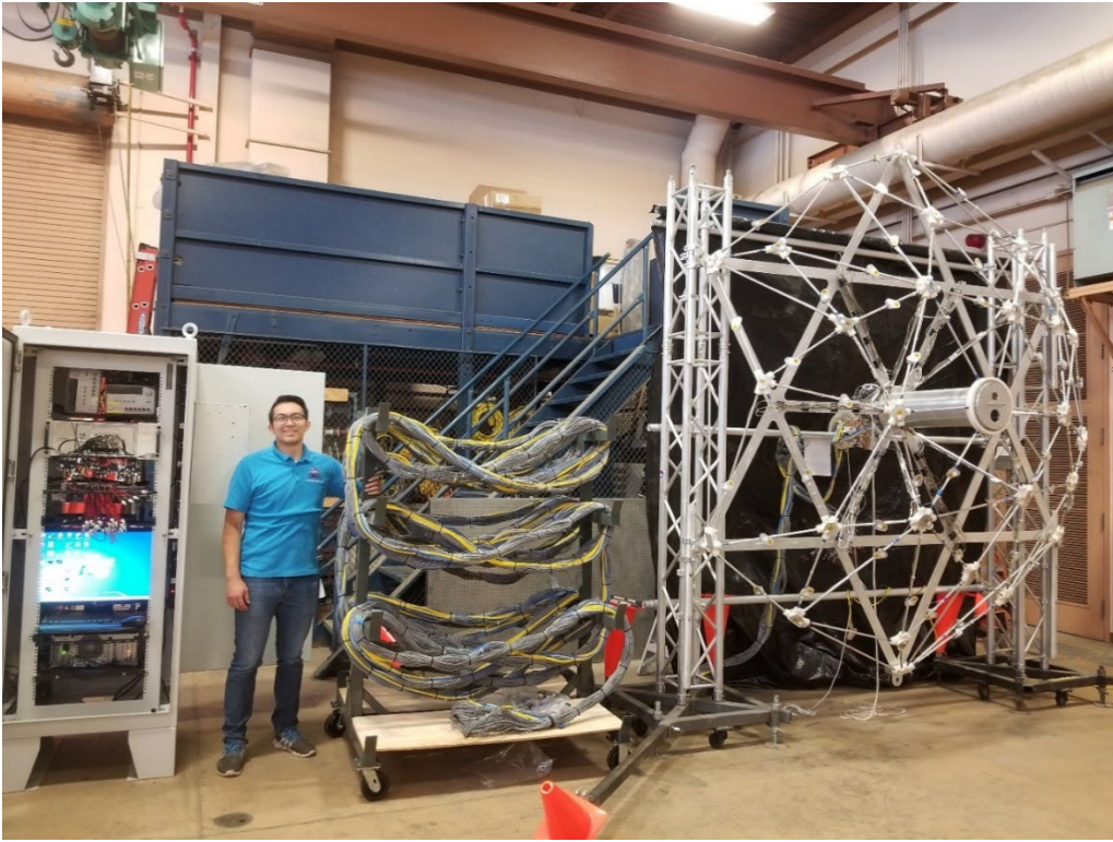
Fig 3. Overall view of the phased array, cable bundle, and data acquisition cabinet.
