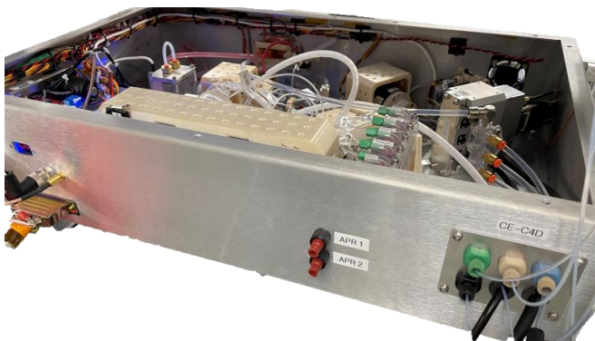
Figure 7. The CE-C 4 D instrument. Left, a table of inorganic species already demonstrated by the CE-C 4 D system. Right, an image of the field portable CE-C 4 D system with its cover off.
