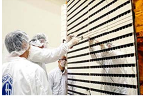
Figure 14.6 Solar panel for the MESSENGER mission, showing that two-thirds of the array area is covered with mirrors, and only one-third of the area (dark stripes in the image) has solar cells. Courtesy NASA.
