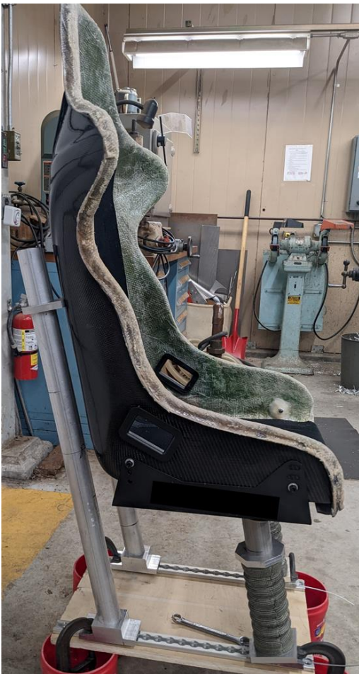
Figure 6 - NASA developed EA seat.
