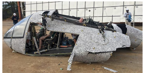
Figure 11 - Post-test damage in the port side.
