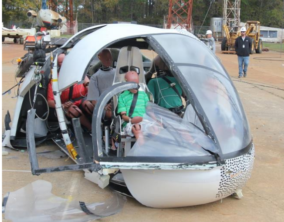
Figure 12 - Post-test damage in the nose section.
