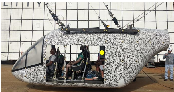
Figure 9 - Pre-test configuration for LPC test article.
