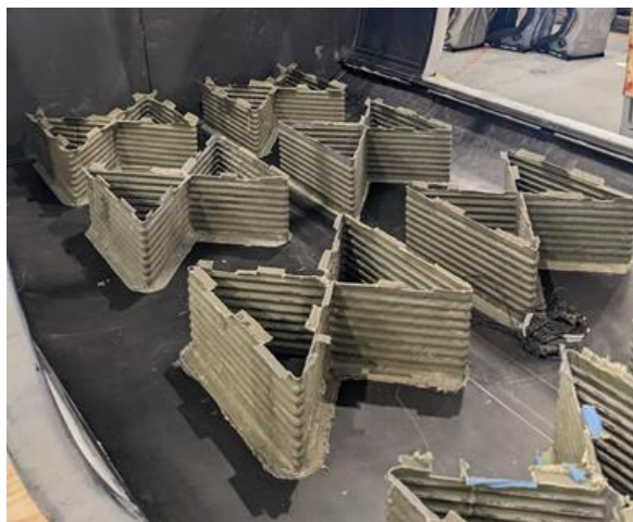
Figure 3 - Energy absorbing subfloor components.
