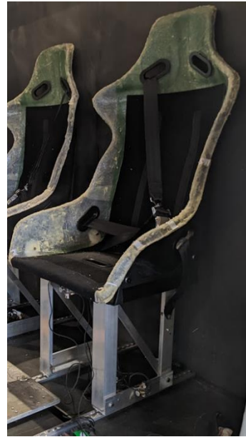
Figure 7 - Composite rigid seat design.
