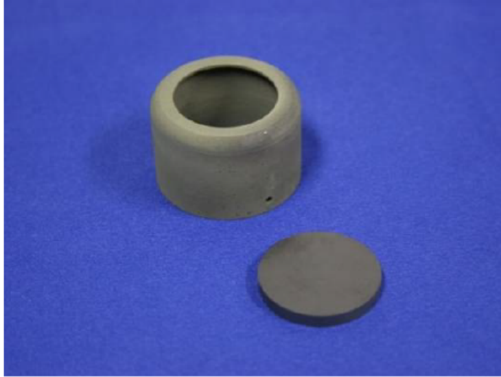
Figure 4.3: A photograph of the SiC probe. Reproduced from Splinter et al. [2011].
