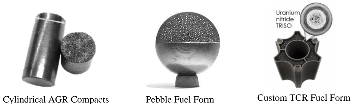
Figure 2-2 Example TRISO based fuel forms developed under the AGR or complimentary DOE advanced reactor / fuel development programs [40, 41, 42]
