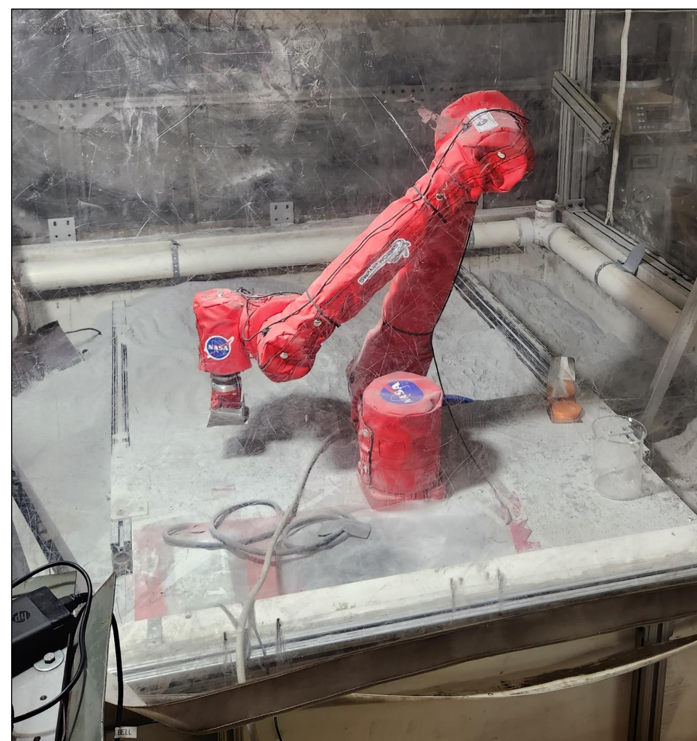
Figure 1. NASA KSC Swamp Works UR10 robotic arm with force-torque sensor in testbed of Exolith Lab Simplified LHS-1 simulant
