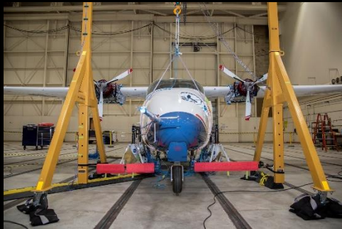
NASA's all-electric X-57 Maxwell prepares for ground vibration testing at NASA's Armstrong Flight Research Center in California. Credits: NASA Photo / Lauren Hughes
