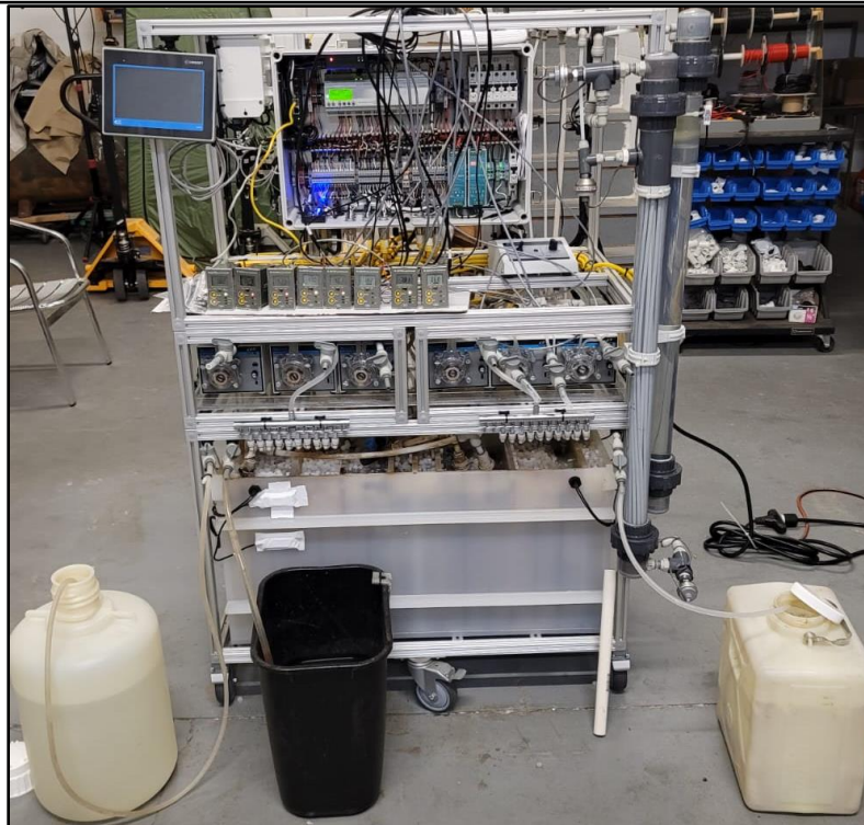
Figure 3. a). Diagram of SAMBR function and operation b.) Fabricated SAMBR system during hydraulic testing. *Patent Pending*
