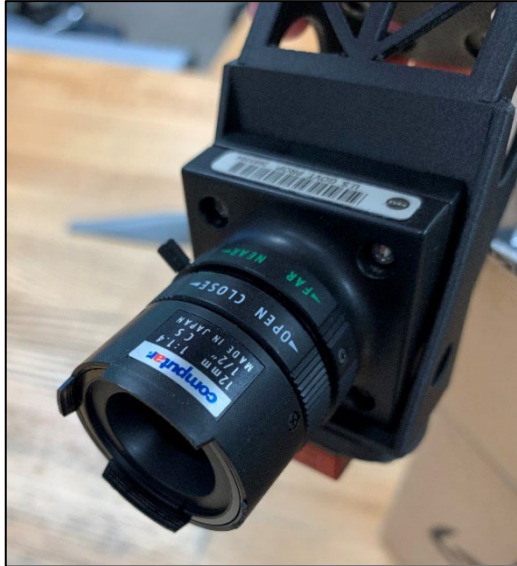
Figure 24 - UI 1250ML Progressive Scan Camera Used for Safe2Ditch Vision Assisted Landing
