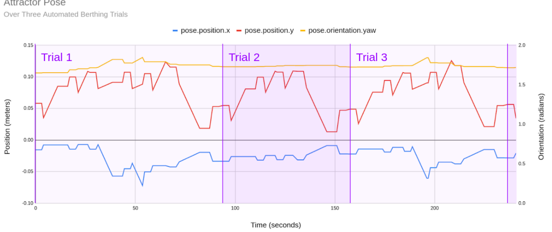
Figure 7: A plot of the attractor position and orientation during three automated berthing operations.
