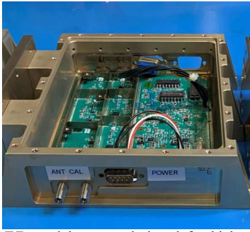
Fig. 5 SESAR's T/R modules were designed for high efficiency, robust performance, compactness and reduced weight while exhibiting optimum system performance. Each module is paired with an antenna subarray to support beamforming operation. The modules also included independent loop back calibration paths.
