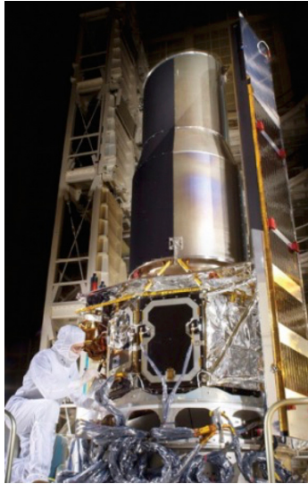
Fig. 3 The assembled Spitzer observatory being prepared for thermal vacuum testing at Lockheed Martin in Sunnyvale, California. The photograph illustrates the key features of the thermal control system up to and including the outer shell of the telescope. These include the chevron-shaped solar panel, the solar panel shield immediately behind it, and the telescope outer shell, with its antisolar side painted black to maximize its infrared emissivity. Also visible between the spacecraft and the outershell is the spacecraft shield, which isolated the outer shell from the spacecraft. Credit: NASA.
