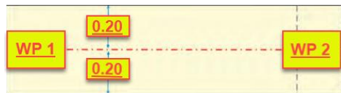
Figure 18. 8260.58 RNP 0.1 track-to-fix waypoint criteria
