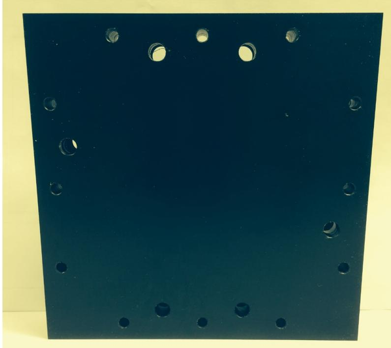
Figure C7.—The 20% Glass-Filled Polycarbonate Endplate.
