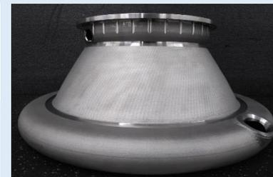
**GRX-810**, high strength, low creep rupture and oxidation at extreme temperatures
