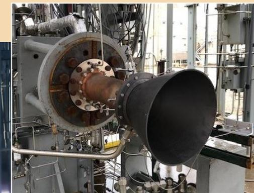
7k-lb<sub>f</sub> GRCop-42 chamber and Composite Nozzle
