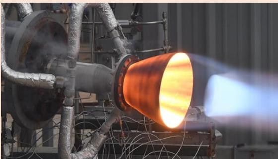
**NASA HR-1**, high strength superalloy for hydrogen environments
