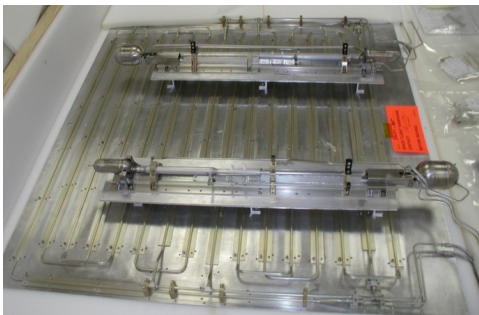
Loop Heat Pipe and Radiator System
