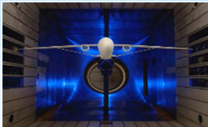
Transonic Truss-Braced Wing ~5-10% fuel burn benefit
