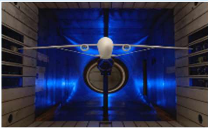
Transonic Truss-Braced Wing ~5-10% fuel burn benefit
