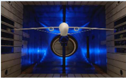
Transonic Truss-Braced Wing ~5-10% fuel burn benefit
