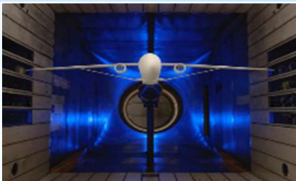
Transonic Truss-Braced Wing ~5-10% fuel burn benefit
