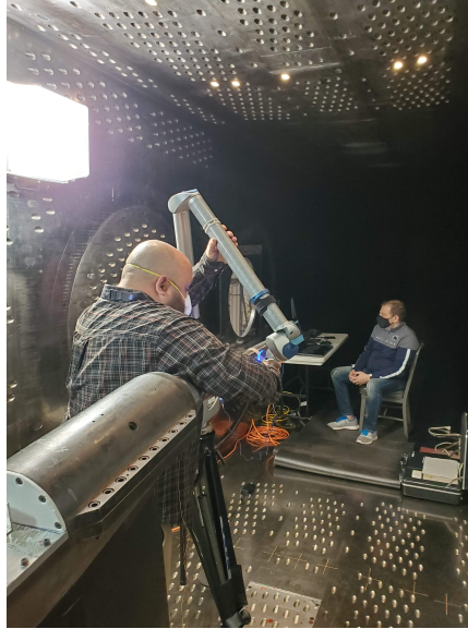
Fig. 17 Faro Arm Coordinate Measuring Machine (CMM) measurements [Source: NASA].
