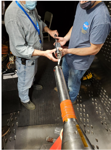
Fig. 10 Installation of the probe into the back part of the sting [Source: NASA].
