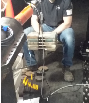
Fig. 22 Weights being loaded on the loading block [Source: NASA].
