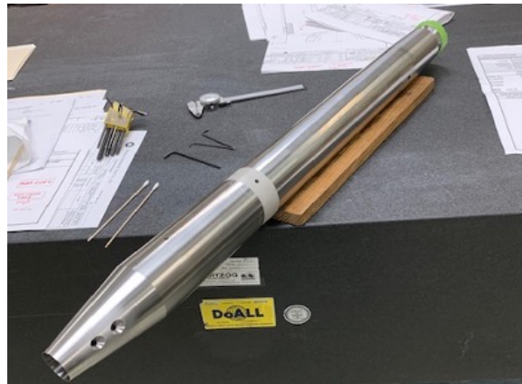
Fig. 9 The sting with the collar between the two halves [Source: MM&T].
