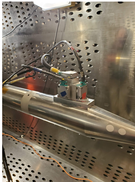
Fig. 23 AMS installed on the sting leveling plate [Source: NASA].
