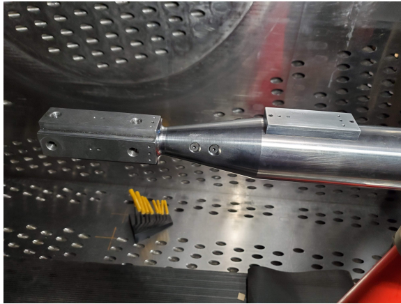
Fig. 19 The loading block and the leveling plate installed on the sting [Source: NASA].
