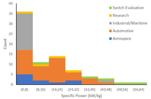
Fig. 1. Distribution of specific powers of the converters included in the database.
