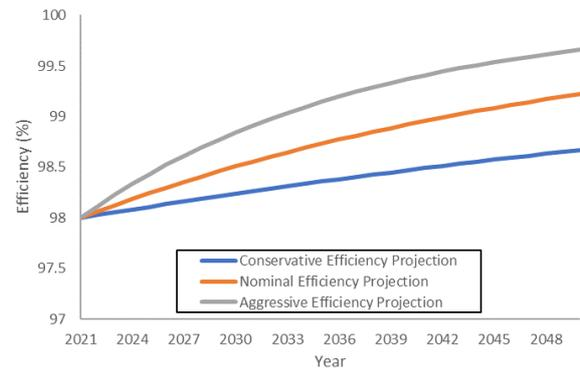
Fig. 8. Efficiency projections.
