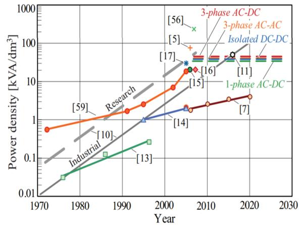
Fig. 3. Historical power converter power density data taken from [10]. Sources in the plot refer to the original paper.
