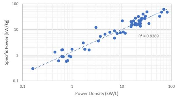
Fig. 4. Relationship between specific power and power density from the converter database [12-38].
