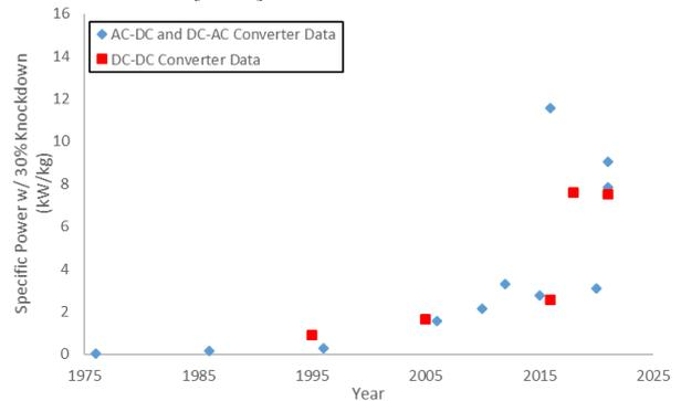
Fig. 5. Converter data used in specific power projections [12-38].
