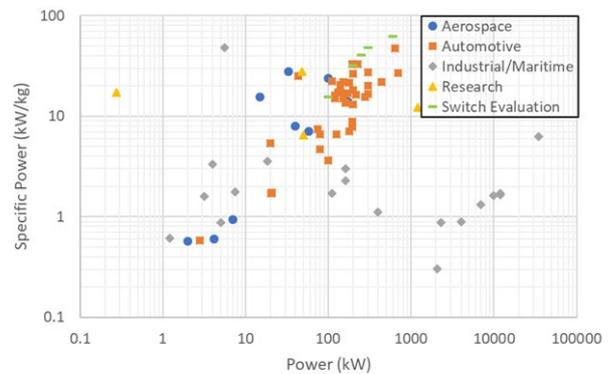
Fig. 2. Specific power vs maximum power of the power converters in the database.
