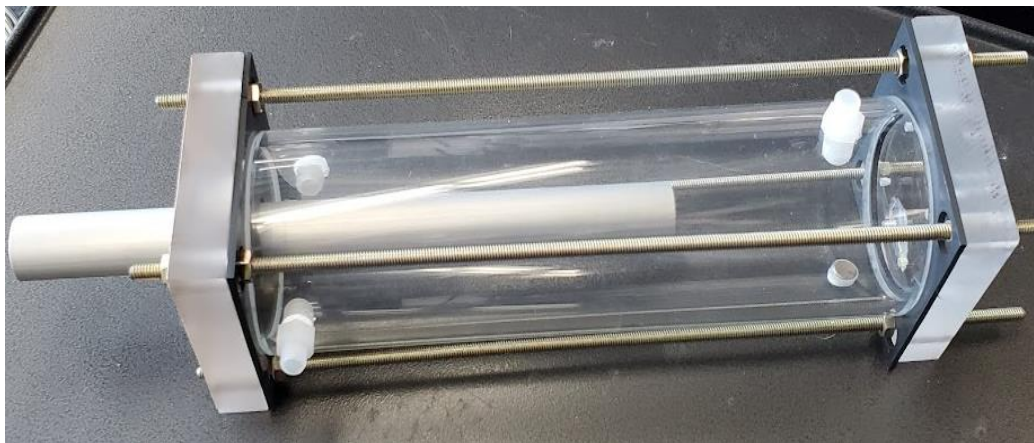
Figure 2.2: Cast acrylic test reactor with anodized aluminum sample. The same dimensions as the PTFE reactor were used in the cast acrylic reactor.
