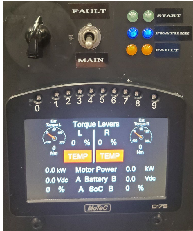
Fig. 6. Multifunction display (MFD); and page selector switches.
