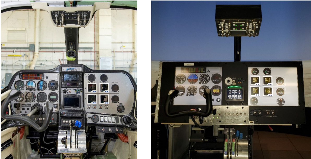
Fig. 4. (left) Aircraft cockpit dashboard; and (right) piloted simulator cockpit dashboard. Photo credit: NASA/Genaro Vavuris.
