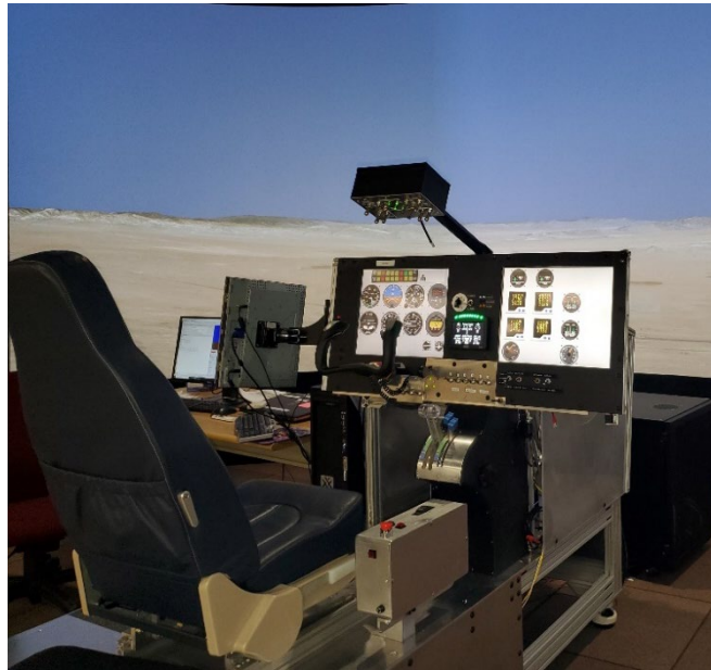
Fig. 3 Piloted simulator cockpit. Pilot seat, controls, switches, out-the-window view, and instrumentation.
