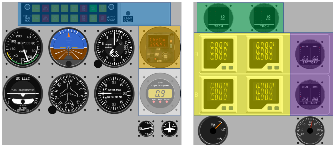
Fig. 5 Head-down display: (left) Panel includes stock P2006T instruments (no shading); radio channel selector (orange shading); annunciator panel (blue shading); and accelerometer (G-meter) (white shading); and (right) panel includes tachometers (green shading); avionic power meters (purple shading); and battery power meters (yellow shading).
