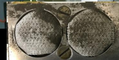
Sample pair after exposure to nitrogen jet
