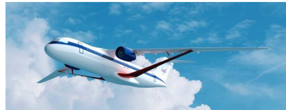
Figure 1. High aspect ratio Transonic Truss-Braced Wing configuration (NASA Photo).
