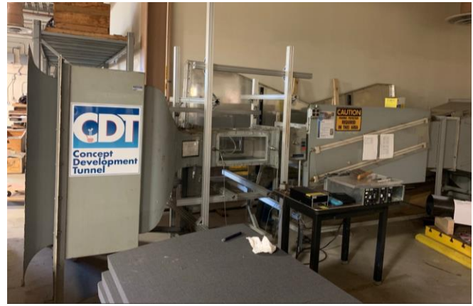
Figure 6. Small wind tunnel used for simple tiltrotor model.
