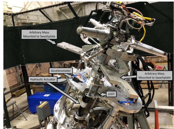
Figure 22. TRAST model with nacelle at 60 degrees, arbitrary masses added to swashplate.
