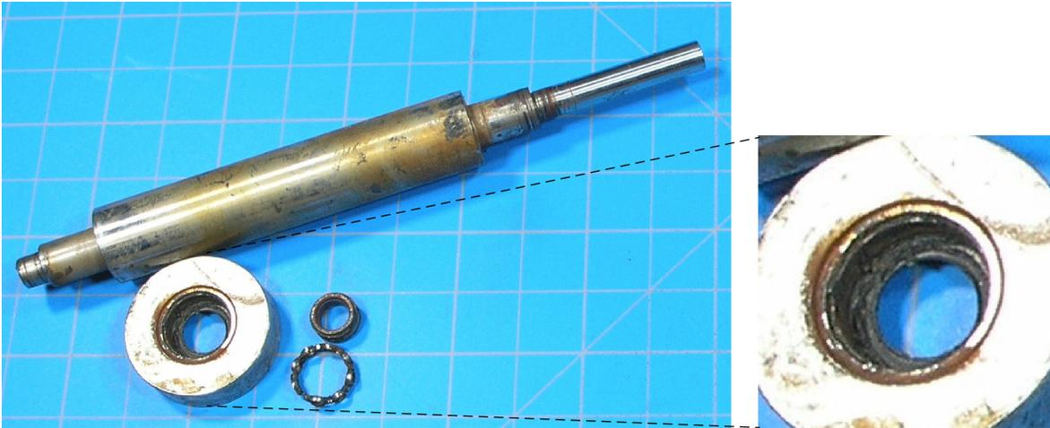
Figure 3.—Spindle and disassembled bearing from 440C 100-h corrosion test.
