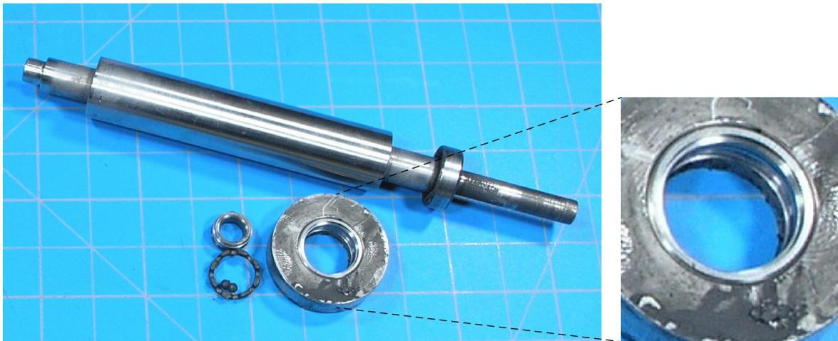
Figure 4.—Spindle and disassembled bearing from NiTi-Hf 100-h corrosion test.
