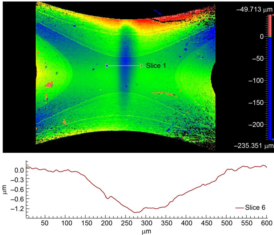
Figure 9.—Sample 3D microscope contour image showing dent and depth measurement.
