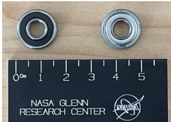
Figure 1.—Representative R4 NiTi-Hf bearings manufactured by two different vendors, one with rubber seals (left), one with metal shields (right).
