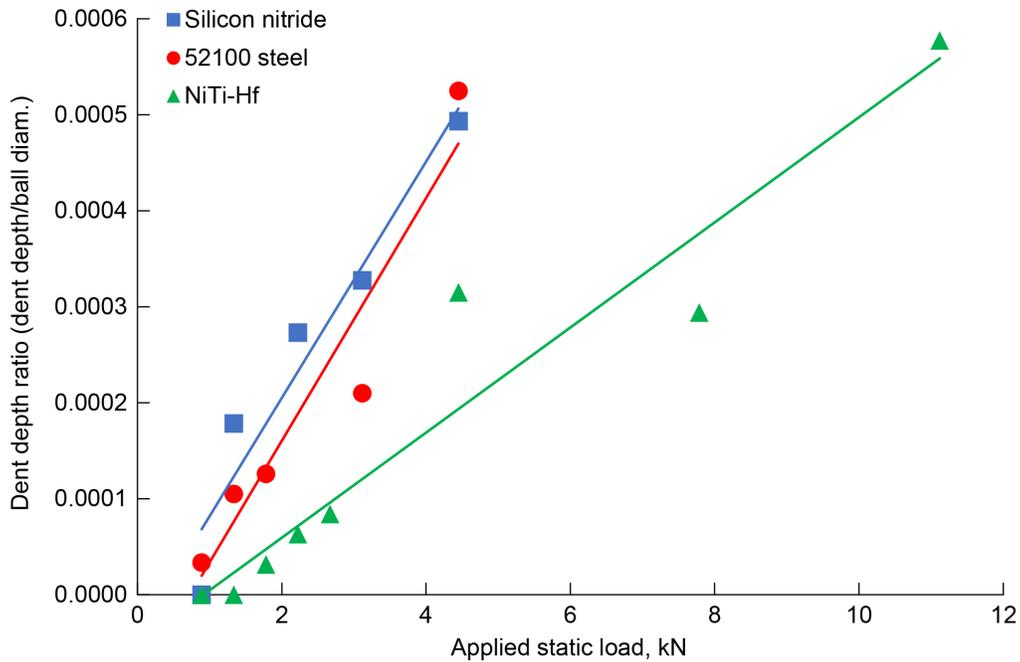
Figure 11.—Dent depth ratio versus applied radial load for Si<sub>3</sub>N<sub>4</sub>, 52100, and NiTi-Hf balls.
