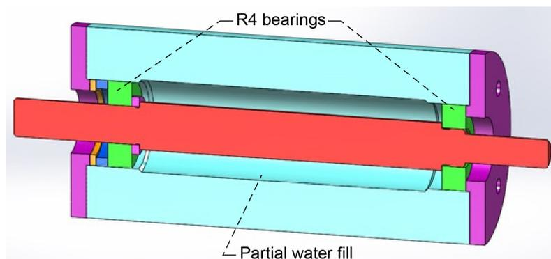
Figure 2.—Cross-sectional schematic of bearing corrosion test setup.
