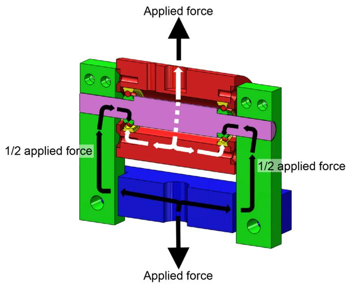
Figure 6.—Cross-sectional schematic of bearing load fixture showing bearing arrangement and load path for applied radial load.
