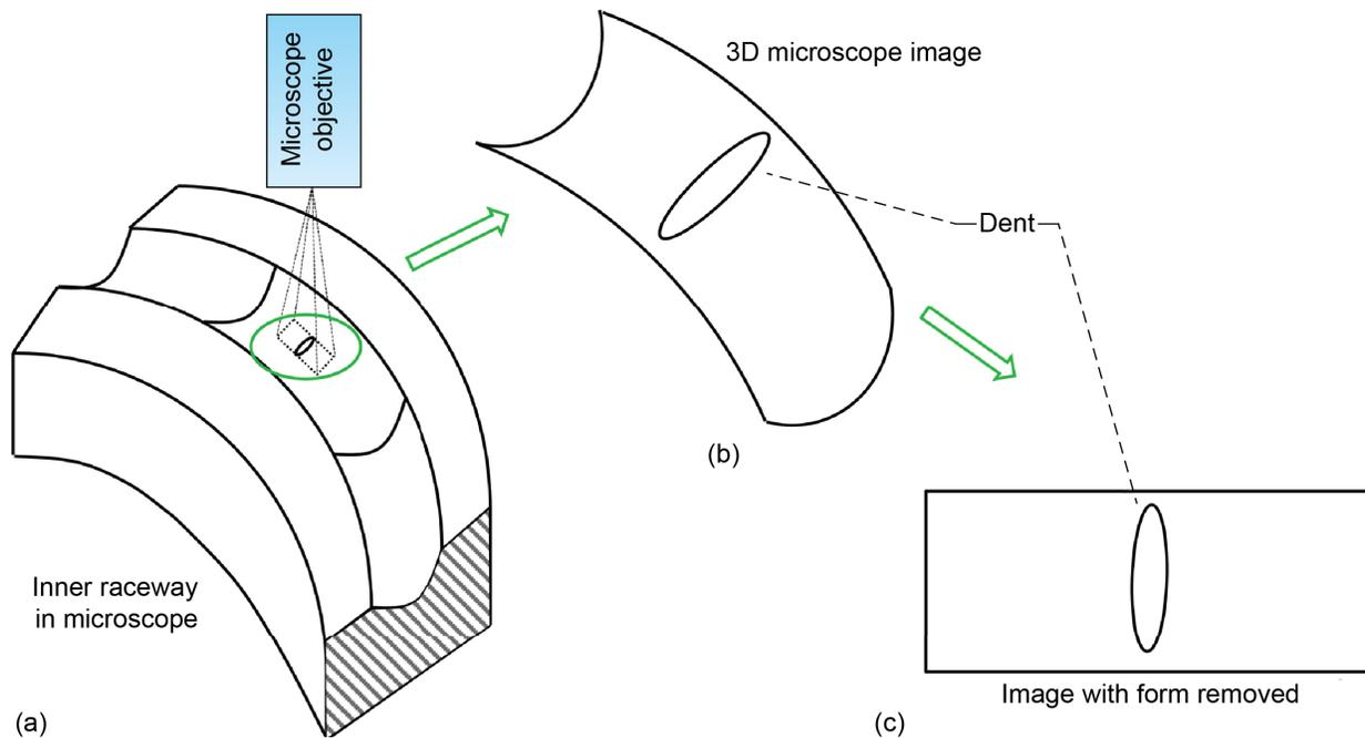
Figure 8.—Conceptualization of 3D microscope imaging technique. (a) Inner raceway under microscope objective. (b) 3D microscope scan with dent near the center of the scan envelope. (c) Flattened image with form removed.
