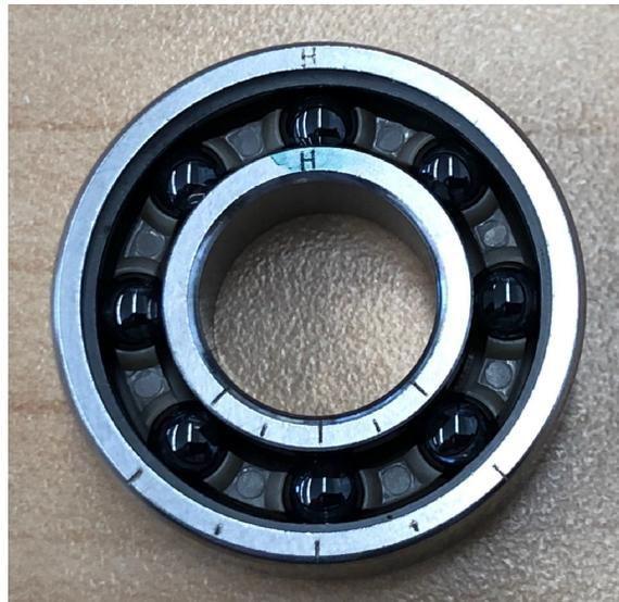
Figure 5.—Hybrid 440C/NiTi-Hf R8 bearing, showing laser etch marks for indexing/positioning.
