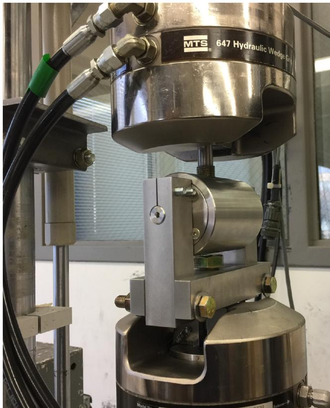
Figure 7.—Bearing load fixture mounted in NASA Glenn's 5-kip axial torsion load frame.
