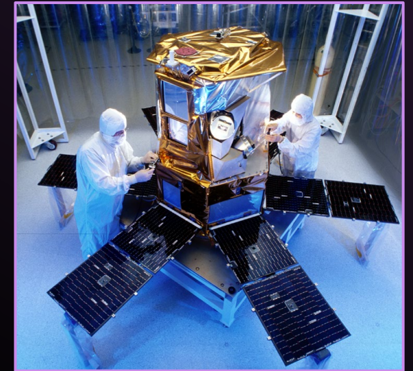
SORCE: 290kg • On an Orbital LEOStar-2 bus
