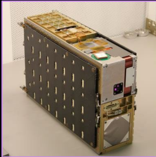
CSIM: 11kg CubeSat • Built by LASP
