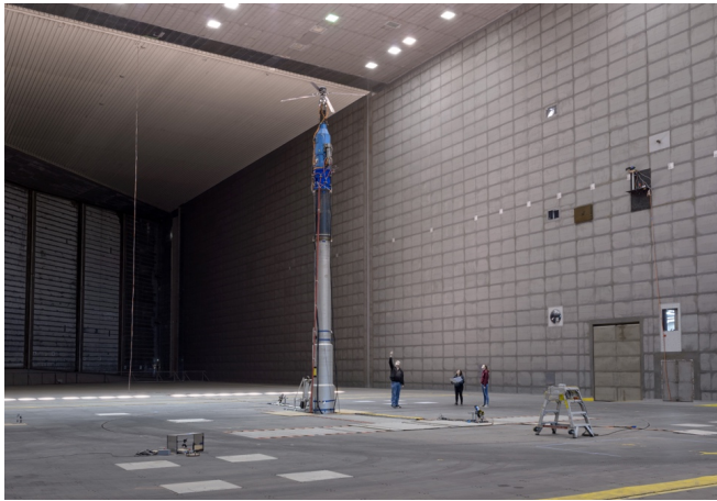
Figure 1. HVAB rotor mounted on ARTS test stand in the NFAC 80- by 120-Foot Wind Tunnel.
