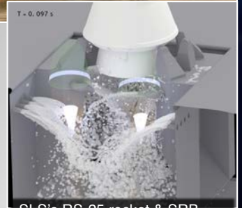
SLS's RS-25 rocket & SRB plume-water interaction simulation
