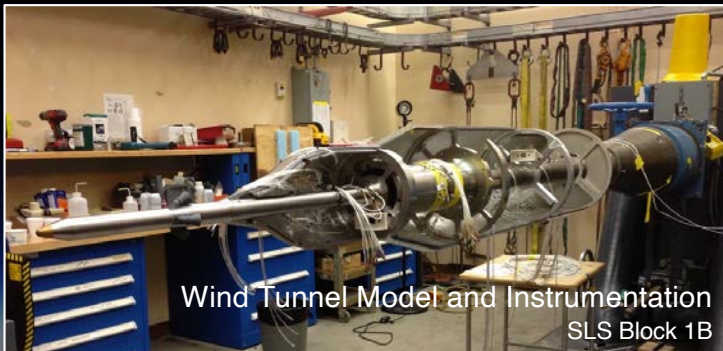
Pressure Sensitive Paint Test Space Launch System
