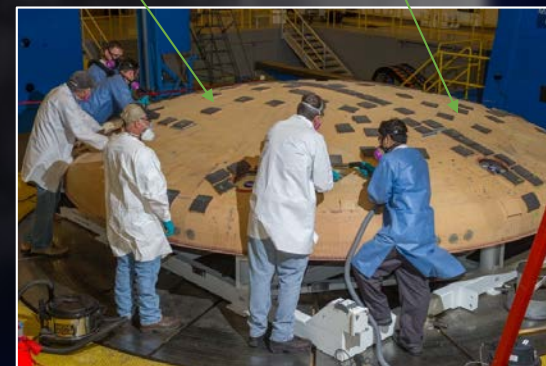
Engineers from Ames Research Center and Marshall Space Flight Center remove Avcoat segments from the surface of the Orion heat shield.
