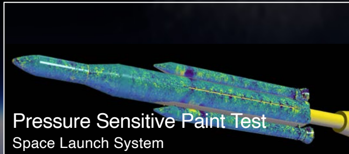
Wind Tunnel Model and Instrumentation SLS Block 1B
