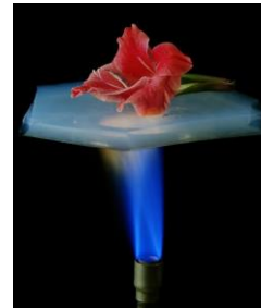
Bunsen burner applied to aerogel
