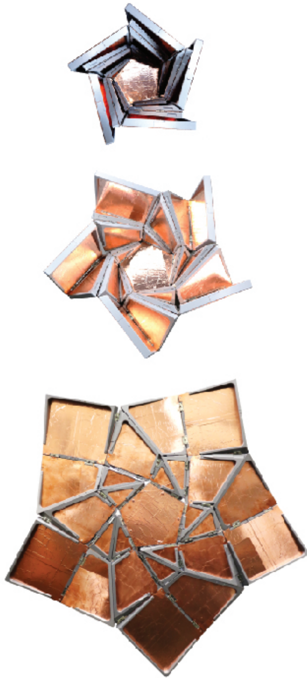
Fig. 10. The flasher array's deployment process is illustrated with stowed, deploying, and fully deployed images. The full prototype unfolds from a small volume to span approximately 1 meter in diameter and provide 0.555\text{m}^2 of working optical area. Fresnel lenses may be replaced with thin copper plating (as shown in this image) for use as a reflectarray.
