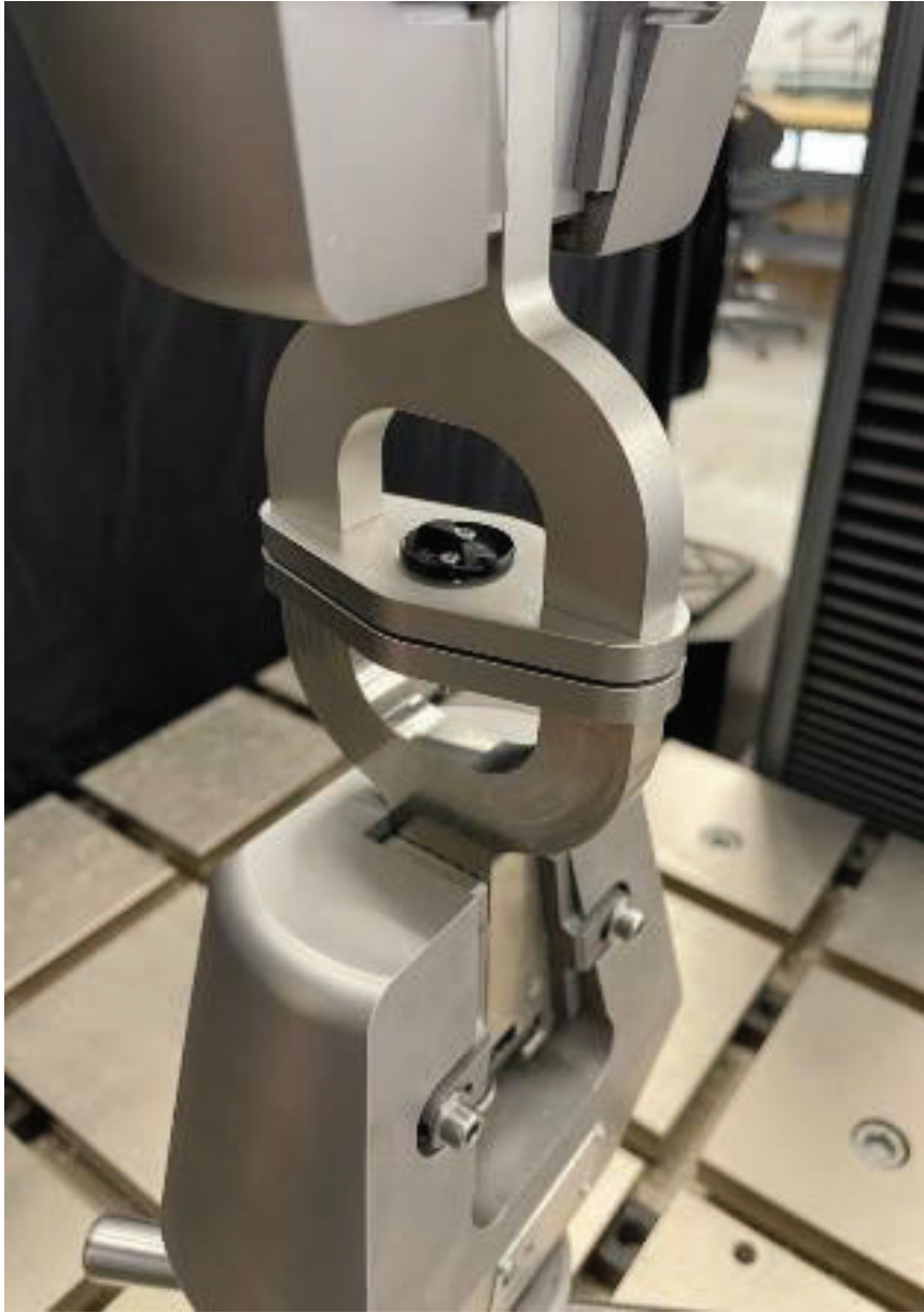
Fig. S5. Fastener tensile testing fixture and set-up.
